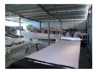
To loft the boat panels a straight line is drawn on the edge of the fabricated panel and the line and marked at 500mm intervals. A square can be used to draw lines perpendicular to the base line. Mark the dimensions given on the plans along the perpendicular lines. Panel pins are nailed at the marks and a flexible baton is bent to create a smooth line. The baton can be made from a narrow piece of plywood the length of the overall panel. Draw the lines onto the peel ply.
